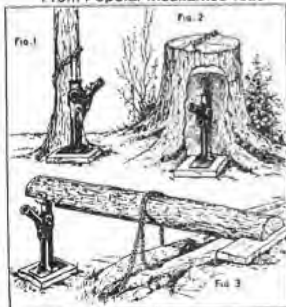
Pulling Up Stumps, Small Trees, and Roots with the Aid of a Track Jack Leaves the Ground Ready for Immediate Plowing
